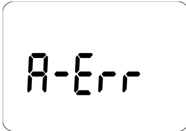
Figure 15 Input terminal warning
