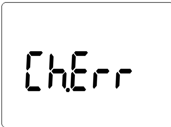
Figure 56 Charge terminal alert
